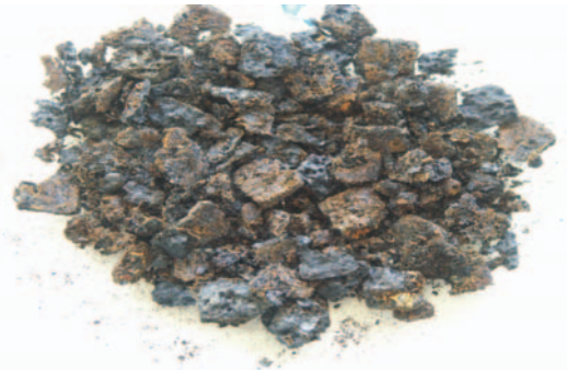
Metallic deposits generated in the cathode compartment of the DFDx cell.
