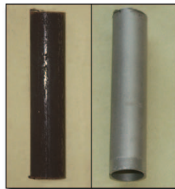
Pre- and post-DFDx processing on a steam generator tube section.
