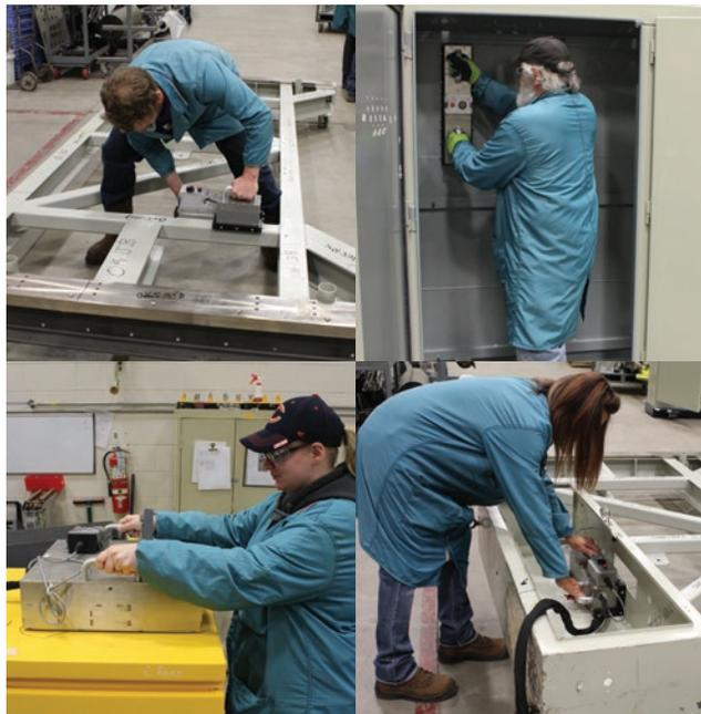
Clockwise from top left: outside corner jig, flat item jig, large area jig, and inside corner jig
