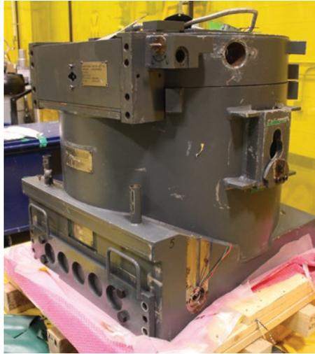
15,000 lb. waste transfer flask (1 of 8) decontaminated and released from a Candu 6 mid-cycle rebuild tool set. 697 crates, 2.5M lbs. of UN2910 and UN2915 materials exported on 69 trucks.
