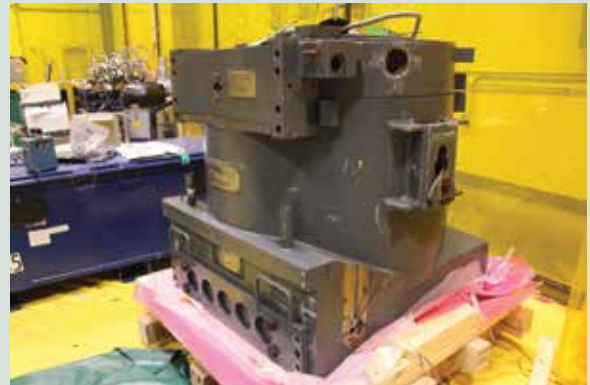
15,000 lb. waste transfer flask (1 of 8) decontaminated and released from a Candu 6 mid-cycle rebuild tool set. 697 crates, 2.4M lbs. exported on 69 trucks.
